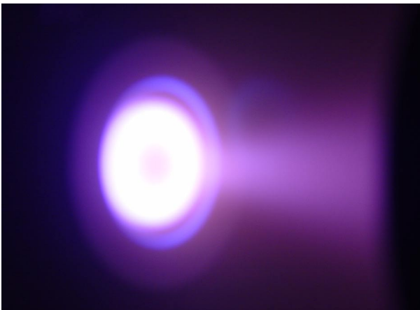
Photograph of a PVD Products 2-inch Titan Magnetron sputter source operating at 500 Watts and 5-mTorr of Argon gas with a Ti target.
