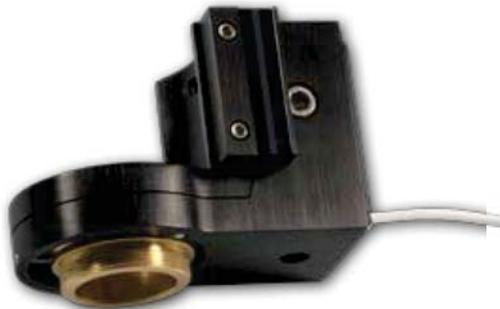
Nano-F100S objective lens nanopositioner is included with the C-Focus™ system. Microscope focus drift is corrected by moving the objective lens in response to feedback from the C-Focus™ sensor system.
