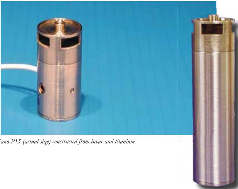
Nano-P15 (actual size) constructed from invar and titanium.
