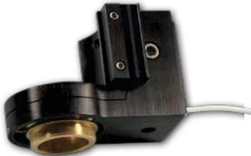
*Nano-F100 objective lens nanopositioner is included with the C-Focus system. Microscope focus drift is corrected by moving the objective lens in response to feedback from the C-Focus sensor system.*
